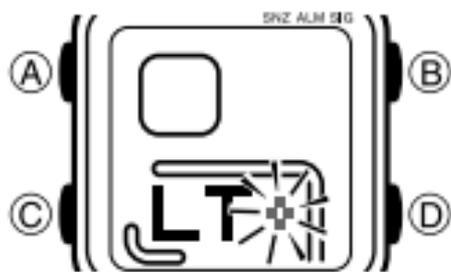
1. In the Timekeeping Mode, hold down (A) until the seconds start to flash, which indicates the setting screen.
