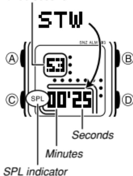
The stopwatch lets you measure elapsed time, split times, and two finishes.
