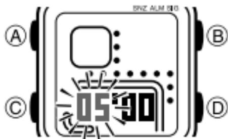
1. While the countdown start time is on the display in the Countdown Timer Mode, hold down (A) until the current countdown start time starts to flash, which indicates the setting screen.
