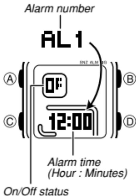
You can set five independent Daily Alarms. When an alarm is turned on, the alarm tone sounds when the alarm time is reached. One of the alarms is a snooze alarm, while the other four are one-time alarms.
