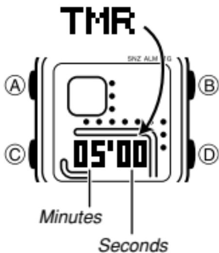
The countdown timer can be set within a range of one minute to 60 minutes. An alarm sounds when the countdown reaches zero. The countdown timer also has an auto-repeat feature and a progress beeper that signals the progress of the countdown.
