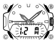
In some cases, such as when the sensor is exposed to wide changes in temperature, the display may show a depth of greater than 1.0 M (4 F) even when you are on the surface. In this case, it is necessary to reset the pressure to "0 M (0 F)". By pressing holding down © and ④ together for at least 1 second, the pressure reading can be reset to "0 M (0 F)". Always perform the above operation on land or on a boat. Do not perform it while in the water.
